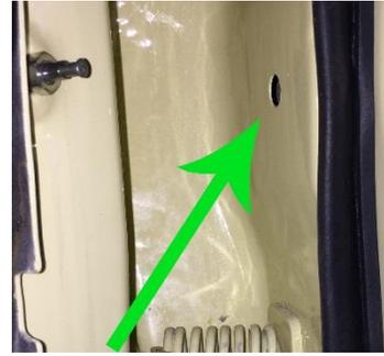
If you do not have the hole in the door you will see a large dimple on the door like the one in this picture. This dimple is stamped from outside the door which can be difficult to drill. The only way to drill this with the door on the car is from the inside of the door but with the dimple going inward keeping a drill bit centered here might be difficult. Do your best, a center punch might be an option if you can get inside the door to do it. Drill a 1 1/8" hole on center with this dimple.
