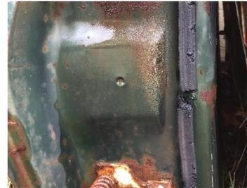
Like the door, the door jam/cowl might already have a small hole drilled. Drill a 1 7/8" hole on center with this hole for the conduit.
